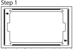
Adhere the adhesive strips on the back of the Surface Mount bracket as shown.
