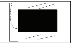
Adhere the backing label to the oposite side of the glass to hide the back of the Surface Mount and iPad.
