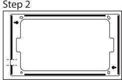
Cut a piece of the adhesive strip where the lightning cable will route behind Surface Mount.
