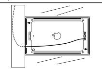
Connect the iPad and place it in the bezel. Attach the bezel to the bracket. Adhere the Surface Mount bracket to the glass close to the channel. Step 5
