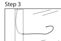
Drill a 3/8" small hole and route the cable down the aluminum channel and out the hole. Make sure there is enough length.
